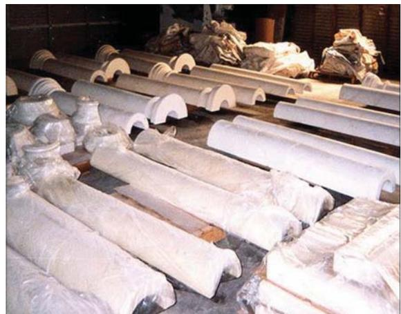
LITEBUILT® LIGHTWEIGHT MASONRY COLUMNS
